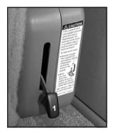
Fold the seatback forward onto the seat cushion by using the lever labeled 1. The seat cannot be removed unless the seatback is folded.
